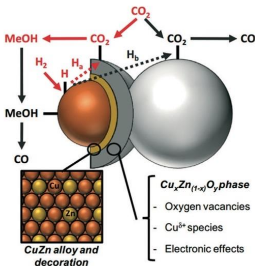
Figure 1.10 General scheme for methanol synthesis over Cu/ZnO-based catalysts. 53
