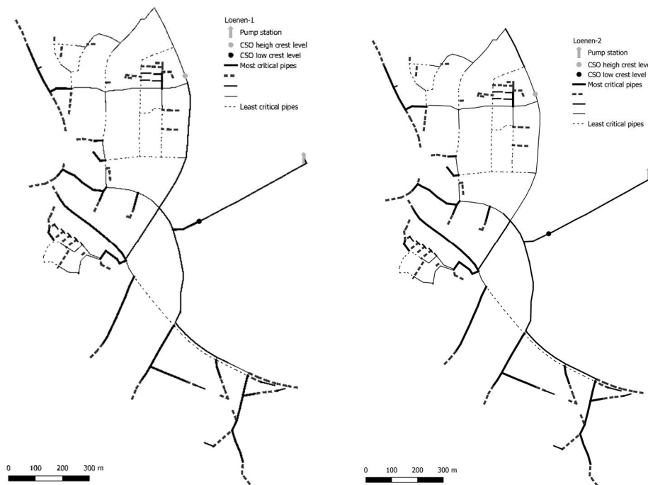
Figure 6.10 Degree of criticality for Loenen-1 (left) and Loenen-2 (right). The darker the lines, the more critical the conduits. Some conduits have the same degree of criticality, but the conduits south of the high overflow structure have a different degree of criticality. In Loenen-2, these conduits are less important because in the case these conduits are blocked the water can flow to the high overflow structure which is not possible in the Loenen-1 system.
