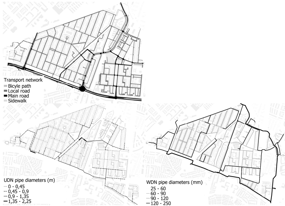
Figure 1.2 Location of elements with the main capacity of the transport network, water distribution network and combined sewer system in Tuindorp, Utrecht, the Netherlands.
