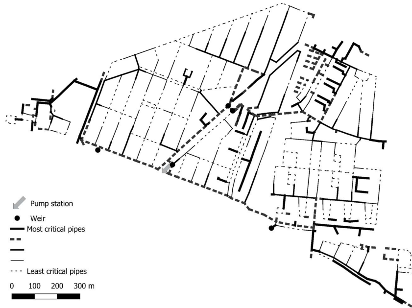
Figure 6.11 Degree of criticality of Tuindorp. The darker the lines, the more critical the conduits.
