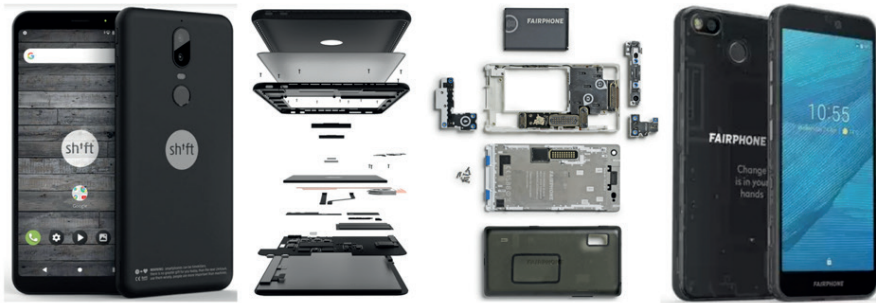
Figure 29. The shift phone (left) and Fairphone are designed modular and can be updated to have new features over time.
