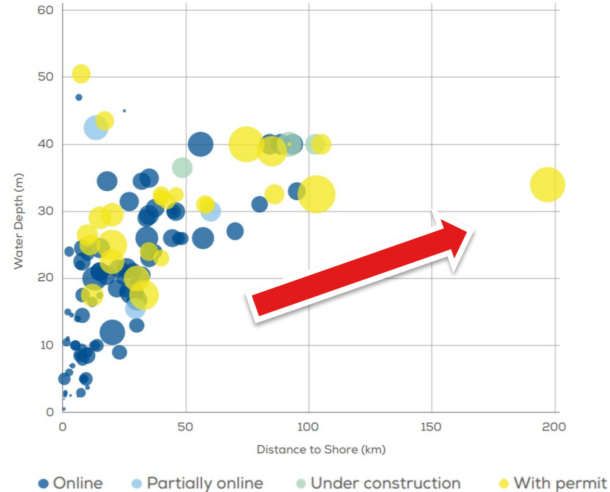
Average water depth and distance to shore of offshore wind farms in Europe [2]
