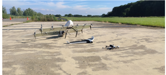
Figure 1: UAV platforms used for the experiments described in this paper. From left to right: Nederdrone (hybrid), Parrot Disco (fixed wing) and a Parrot Bebop2 (rotorcraft).
