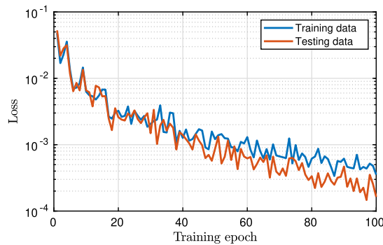
Fig. 11. Synthetic datasets: Training loss calculated from training and testing data sets over 100 training epochs.
