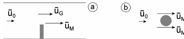
Figure 3-16 Definition of velocities in relation to K_v
