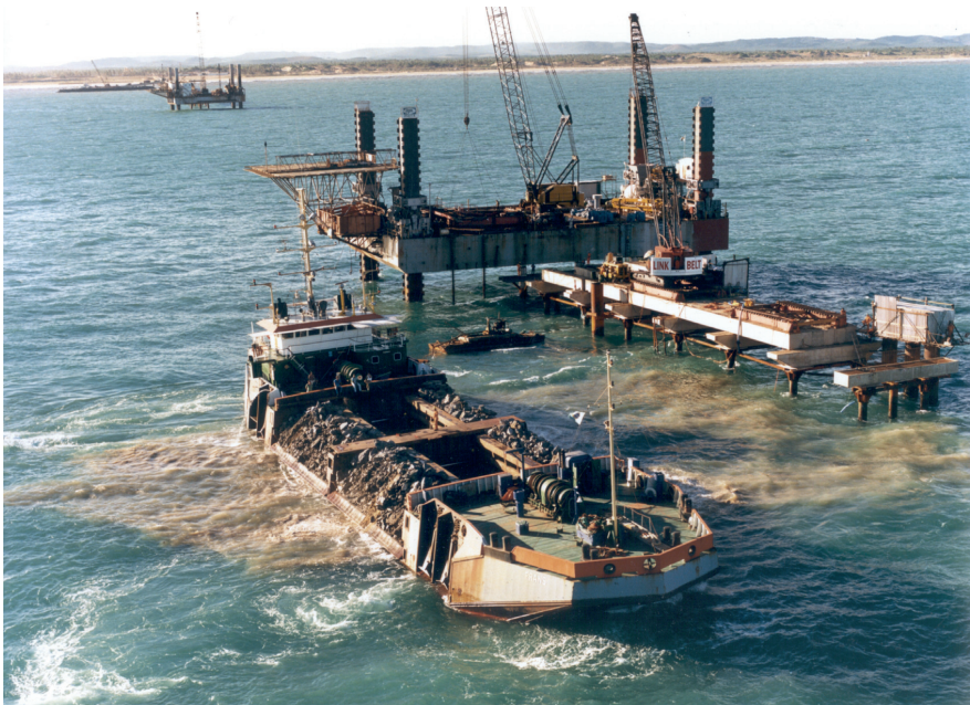
Figure 13-5 Side stone dumping vessel (Boskalis)
