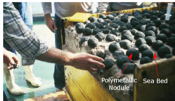
Figure 1. Undisturbed nodule-sediment sample demonstrating the burial of polymetallic nodules (Museum National d’Histoire Naturelle Box Corer [11]).
