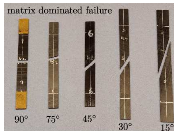
Figure 1. Fractured UD composite laminates under constant strain-rate, for different off-axis angles
