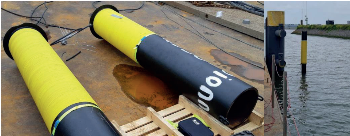
Figure 2. The measuring setup used for a field test in the Botlek, Rotterdam, the Netherlands. Left: a picture of two steel mantels with a fibre optical cable partially wrapped around them to form a receiver array for the experiment. Right: One of the sensing mantels is lowered onto a massive steel pole for continuous monitoring.
