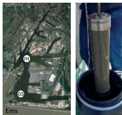
Figure 1. Investigation area and sampling locations IH and GS (left, © Google Earth), Beeker sampler (right)
