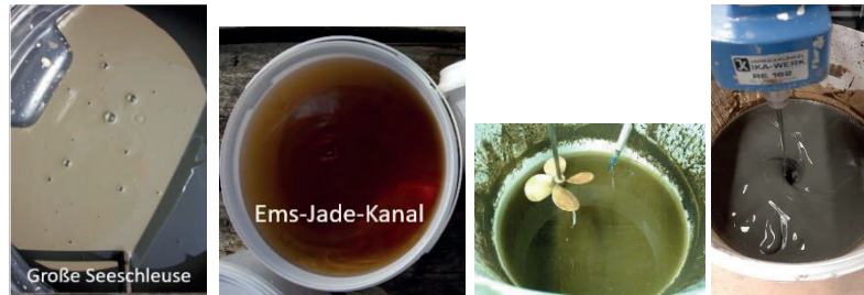
Figure 2. Fluid mud and fresh water sample (left), shearing with vane (right)
