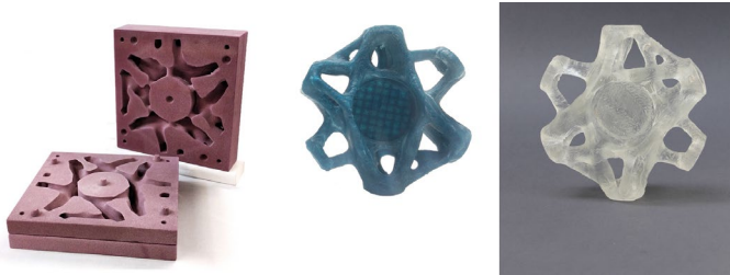
Fig.8: Left: 3D-printed sand moulds produced by ExOne; middle: 3D-printed wax positive model. right: cast glass prototype of the grid-shell node made by the wax model and a silica-plaster mould
