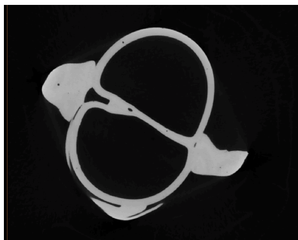
Figure 4. Horizontal X-ray \mu -CT cross section of object 1154 showing the handles at the vessel's sides, the diaphragm, and the onset of the decorative glass trail at the bottom of the image
