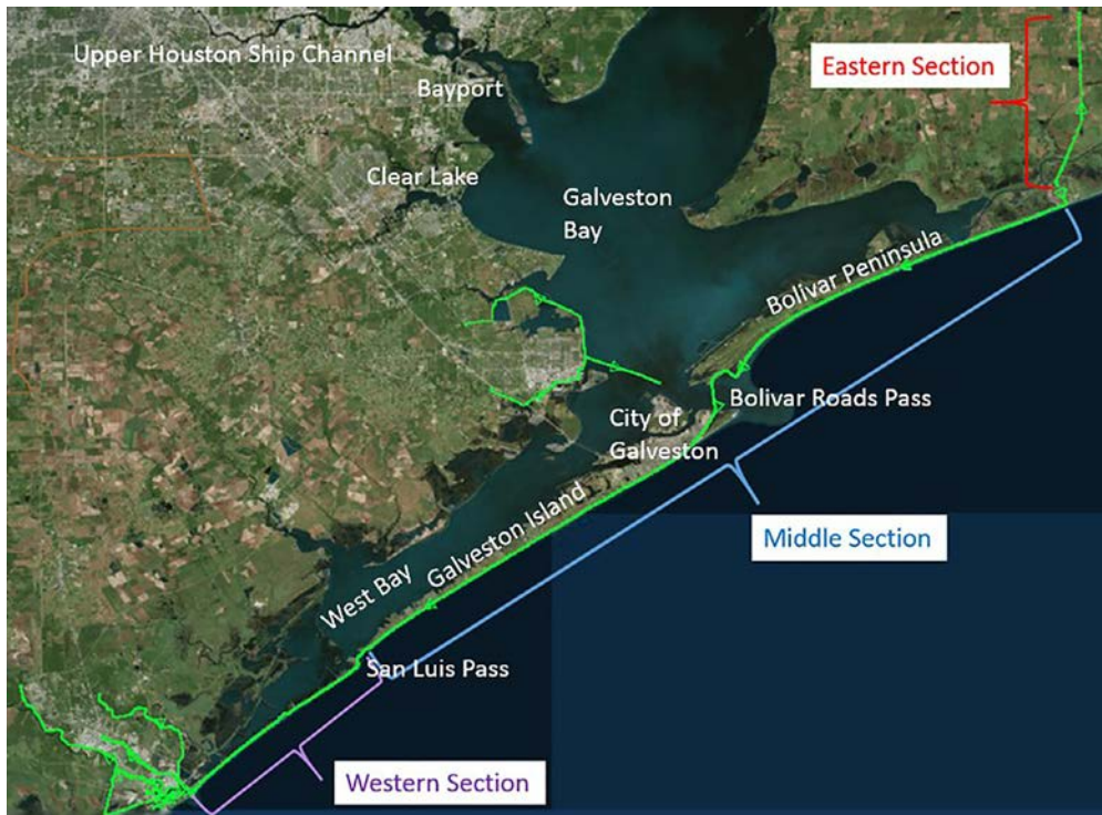
Fig. 1 Location map for the Houston-Galveston region, and footprint of the Ike Dike coastal spine concept.
