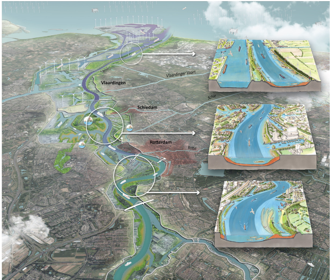
Fig. 3 The Rhine mouth as an estuary, by making the riverbed of the New Waterway more shallow and wider. (Drawing by Dirk Oomen en Peter Veldt (Bureau Strooming).)
