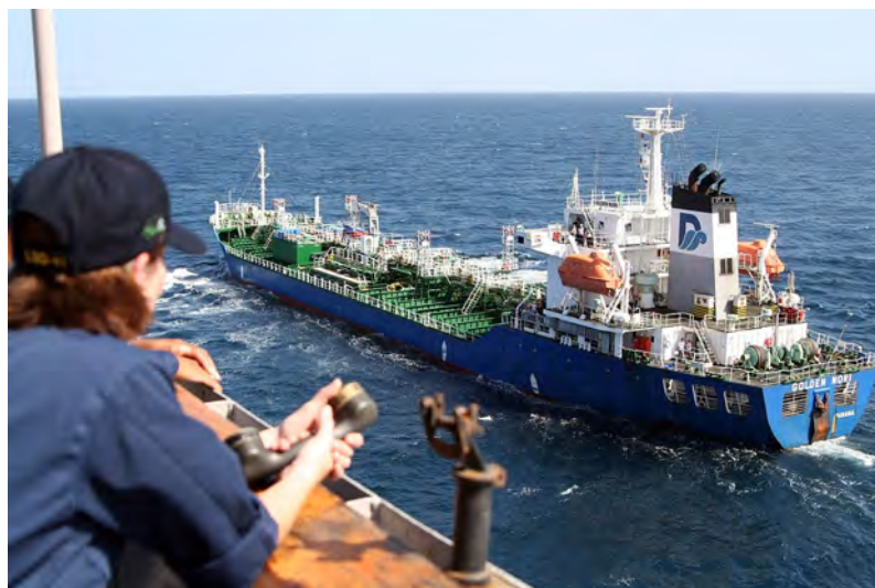
Figure 5.13: Chemical tanker at sea; note the transverse stiffeners on deck (GULF OF ADEN (Dec. 13, 2007) by U.S. Navy photo by Cmdr. M. Junge is licenced under CC0 1.0).
