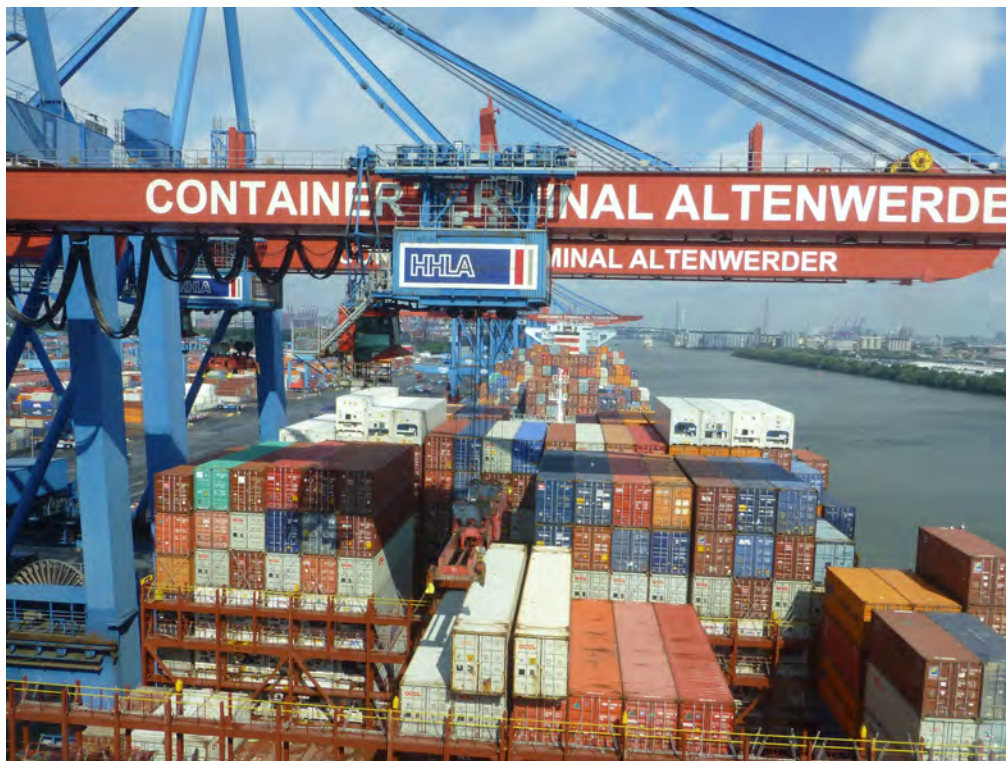
Figure 4.15: Post Panamax STS crane at container terminal Altenwerder, Hamburg, Germany (by www.hippopx.com is licenced under CC0 1.0).
