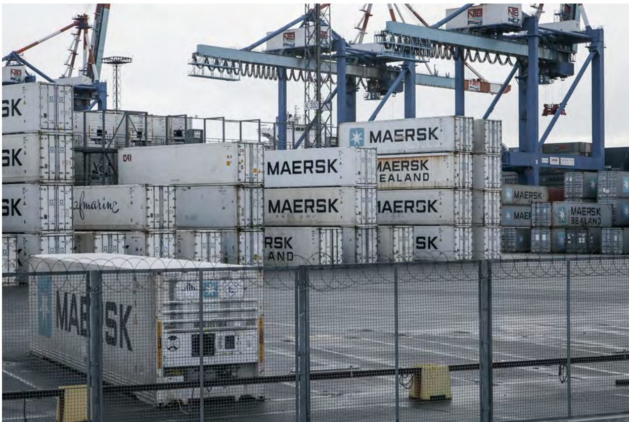
Figure 4.11: Reefer racks in a container storage (by Stefan Georgi is licenced under CC BY-NC-SA 2.0).
