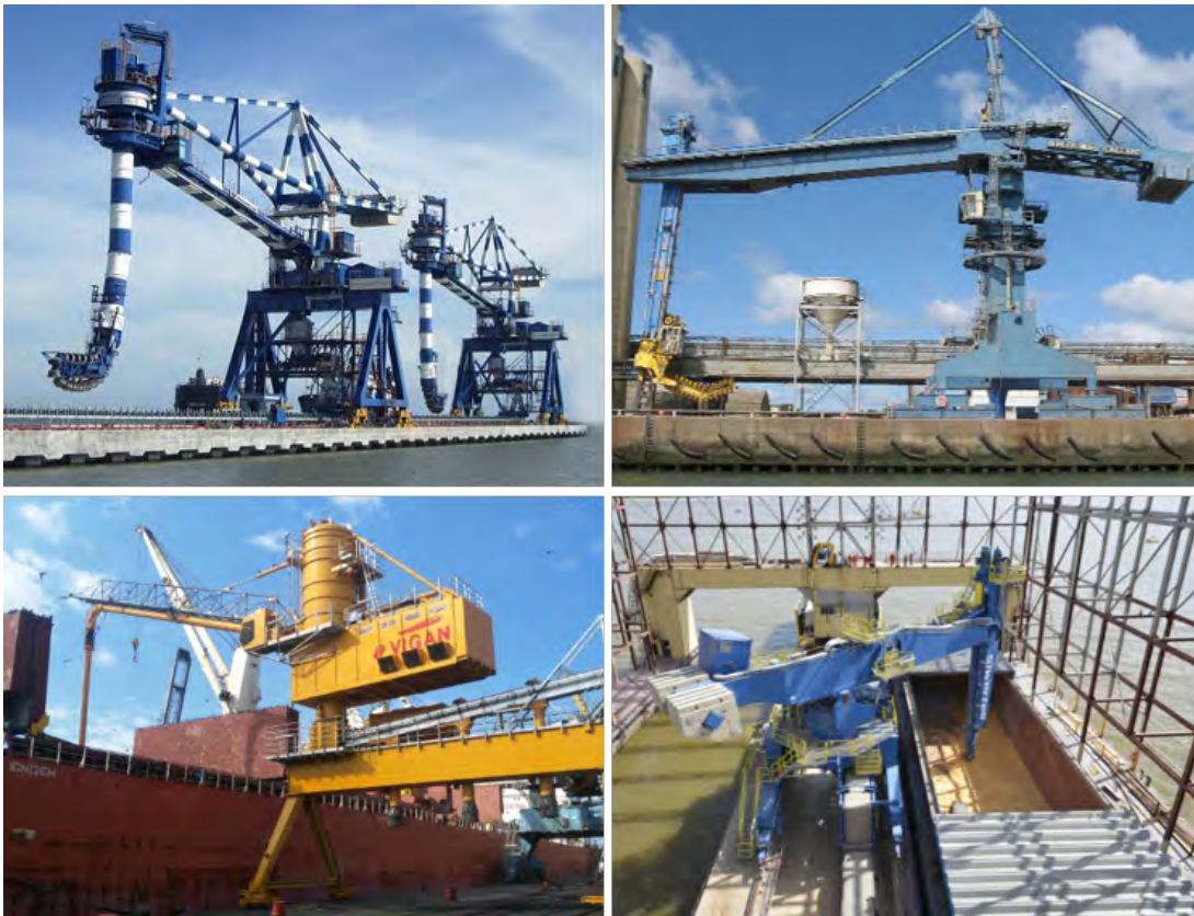
Figure 5.22: Continuous unloaders; top left: bucket elevator type; top right: chain type; bottom left: pneumatic type; bottom right: screw type (images by PIANC, 2019b , are licensed under CC BY-NC-SA 4.0, Port-de-commerce-de-Lorient by Pline is licenced under CC BY SA 3.0).
