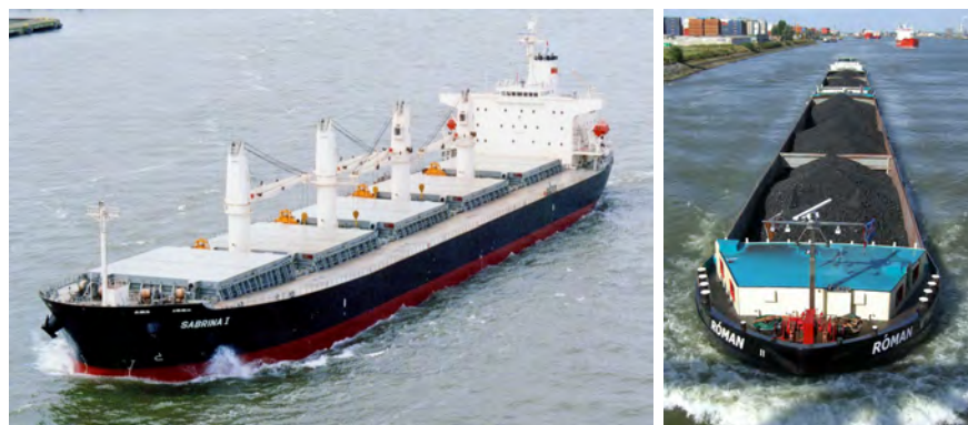
Figure 1.28: Dry bulk carriers; left: Sea-going ( Sabrina I cropped by Nsandel is licenced under CC0 1.0); right: Inland ( Barge Ship Boat by needpix.com is licenced under CC0 1.0).
