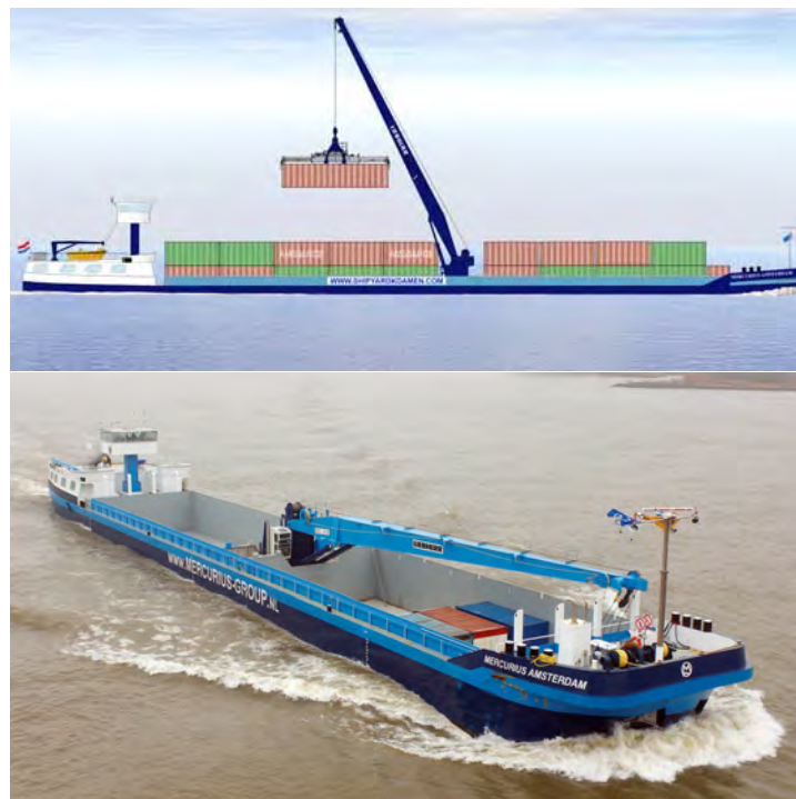
Figure 1.25: Crane barge with its own crane ( MCKS Mercurius by Mercurius Group is licenced under CC BY-NC-SA 4.0).
