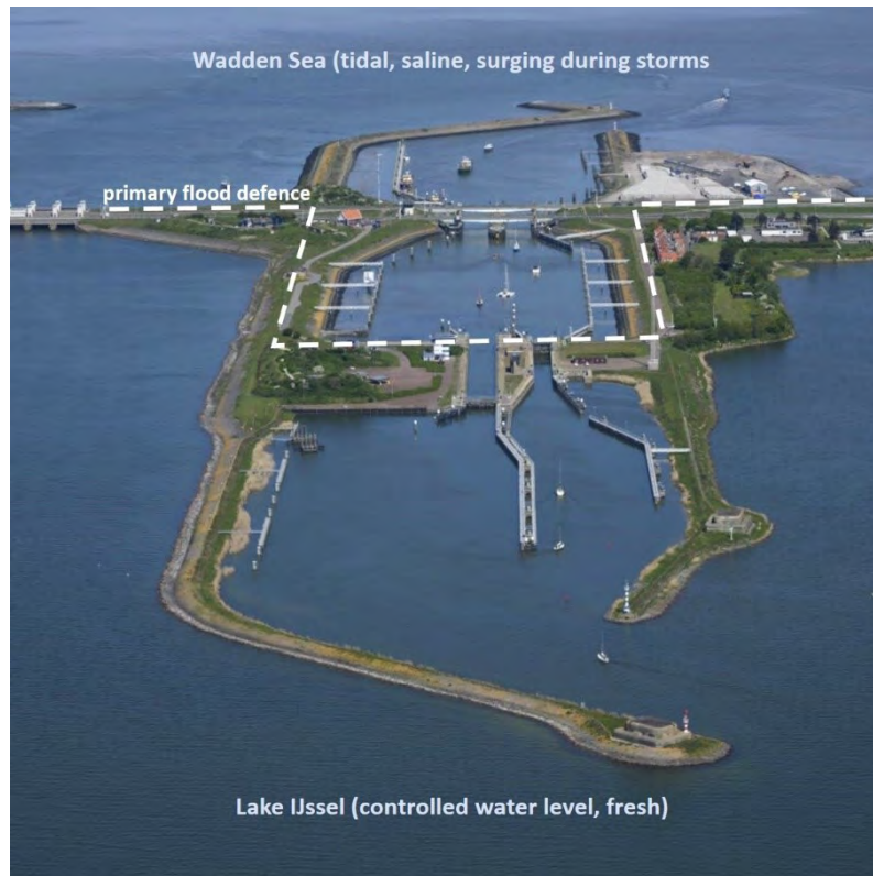
Figure 3.24: Navigation locks in the Afsluitdijk at Kornwerderzand (“Afsluitdijk overview prior to project start” by Royal Van Oord is licensed under CC BY-NC-SA 4.0).
