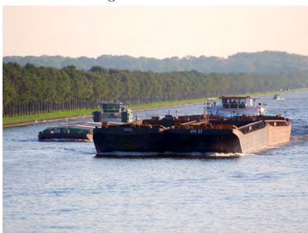
4-barge push-tow unit CEMT-class VIb
