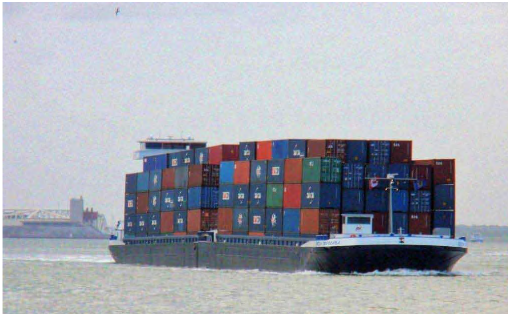
Figure 1.24: The coupled unit Ursa Montana transports 712 TEU (400 × 40-foot high cube containers) (from binnenvaartkrant.nl , “800 TEU in één keer”, Copyright by Binnenvaartkrant).
