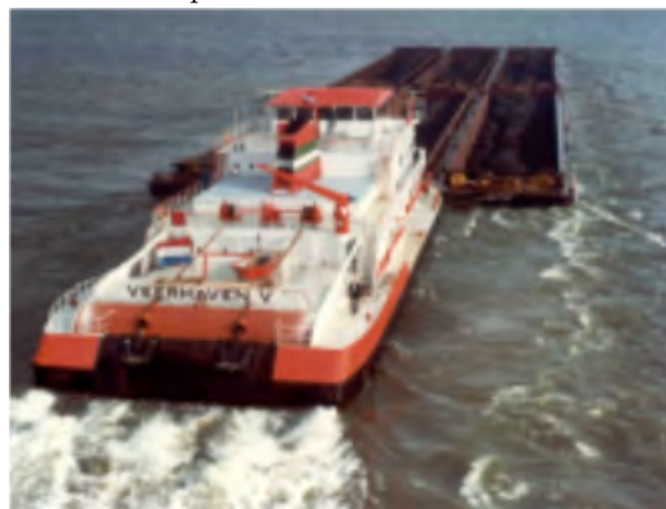
6-barge push-tow unit CEMT-class VIIa
