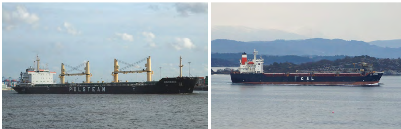
Figure 5.18: Dry bulk carriers with on-board unloading equipment; left: geared Handysize carrier ( Polish Bulk Carrier Kociewie in the Port of Hamburg by Buonasera is licenced under CC BY-SA 3.0 ); right: self-unloader ( CSL Trimnes by Cavernia is licenced under CC BY-SA 4.0 ).
