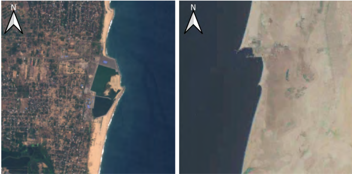
Figure 2.24: Left: Harbour siltation, Oluwil Port, Sri Lanka; right: updrift accretion, downdrift erosion, Port of Nouakchott, Mauritania. Images from Sentinel-2 cloudless by EOX IT Services GmbH are licensed under CC BY 4.0.
