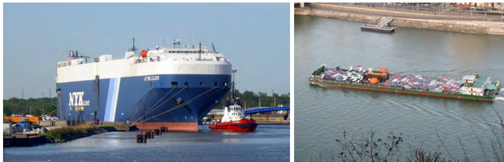
Figure 1.31: Car-carriers; left: Sea-going ( Car carrier Artemis Leader by Tvabutzku1234 is licenced under CC0 1.0); right: Inland ( Barge with cars by Hu Totya is licenced under CC BY-SA 4.0).
