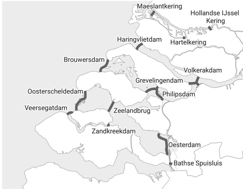
Figure E.7: Delta Works. The Eastern Scheldt, Grevelingen and Haringvliet are (semi-)closed off by the Oosterscheldedam , Brouwersdam and Haringvlietdam , respectively.
