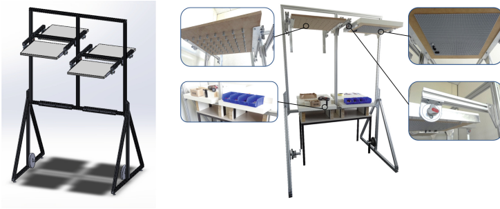
Fig. 1. 3D-CAD drawing of the designed test station (left) and completed test station (right) with enlarged threaded plate, base plate for plug-in test, angle adjustment and tray.
