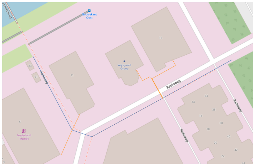
Fig. 11. Selected pipe segments from the sewage network in Almere. Blue: main sewage pipes, orange: home connections.
