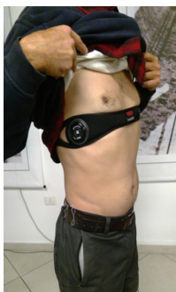
Fig. 4. A worker equipped with Zephyr Bioharness 3
