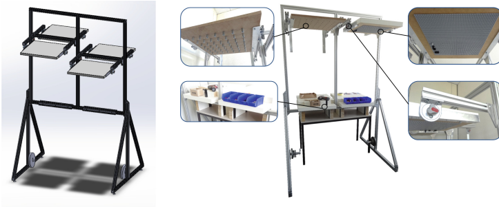
Fig. 1. 3D-CAD drawing of the designed test station (left) and completed test station (right) with enlarged threaded plate, base plate for plug-in test, angle adjustment and tray.
