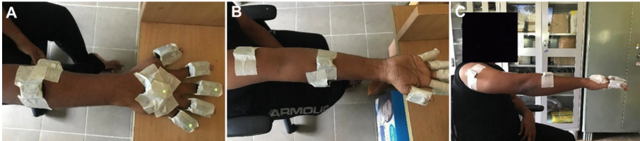
Fig. 2. A, B, C – Accelerometer /EMG sensor placements.
