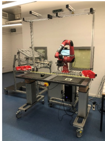
Fig. 1. Workstation for gear assembly.
