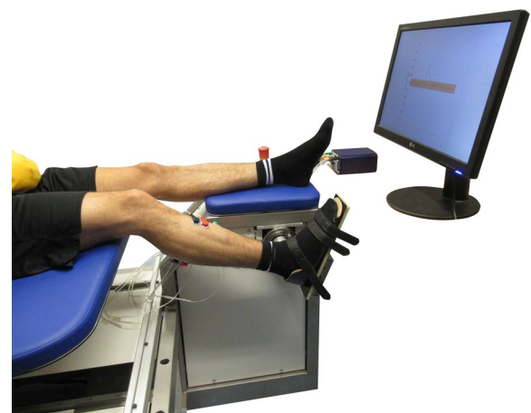
Fig. 1 Experimental Setup. Participants were seated on an adjustable chair for the instrumented evaluations. The manipulator connected to the adjustable chair applied dorsiflexion, ramp-and-hold perturbations around the ankle joint, while measuring the biomechanical response. If the left foot was measured, the right leg was supported with a right lower leg support inserted into the chair frame (not shown)
