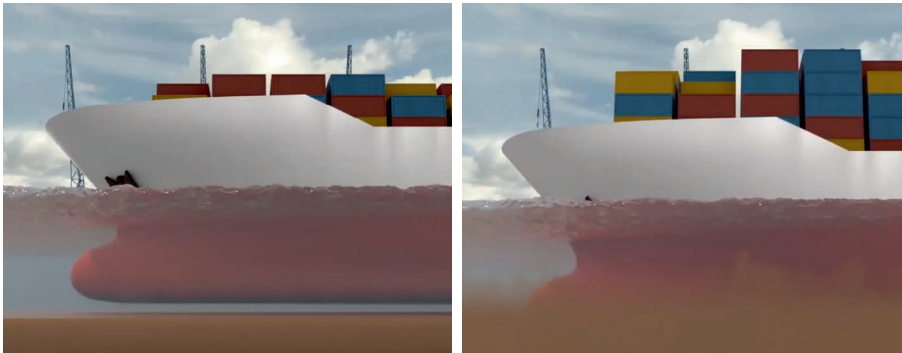
Figure 1.1: A container ship moving above (left) and through (right) a mud layer (snapshots from do] www.youtube.com/watch?v=LSbQhUJMBJw ).
