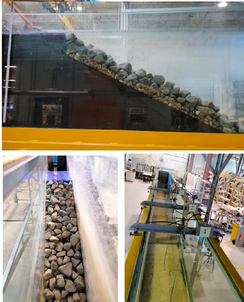
Fig. 3. Longitudinal cross-section of the flume of Griffith University (top); the picture of the constructed model (middle and bottom left); wave gauges (bottom right).
