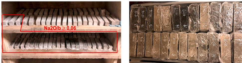
(a) Standard curing condition (95 % relative humidity, 20±2 °C)
