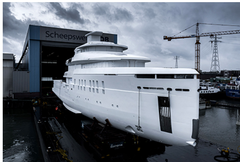
Figure 6. Vertical bow example.
