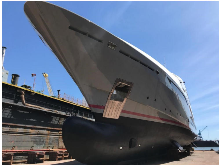
Figure 4. Conventional bow with bulb example.
