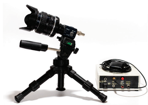
Figure 1. Example (A) of a camera system used by ISO’s: the camera setup of station 4353 in Leiden, the Netherlands, operated by M. Langbroek. This is a WATEC 902H2 Supreme Low Light Level CCTV camera, with time management by GPSBoxsprite-2 GPS time inserter. The lens shown is a Pentax 1.2/50 mm lens, but a Samyang 1.4/85 mm and a Samyang 2.0/135 mm lens are used as well..
