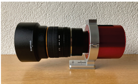
Figure 2. Example (B) of a camera system used by ISO's: the camera setup of station 4171 in Dwingeloo, the Netherlands, operated by C. Bassa. This is a ZWO ASI 1600MM PRO CMOS camera, fitted with a Samyang 1.4/85 mm lens.
