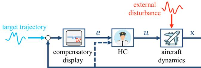
Fig. 3. The pitch angle compensatory tracking task.
