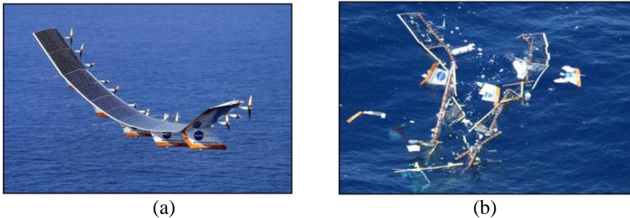
Figure 2.2: The break of NASA's Helios wing. (a) A photo of NASA's Helios wing. (b) A photo of the break of the wing. [18]
