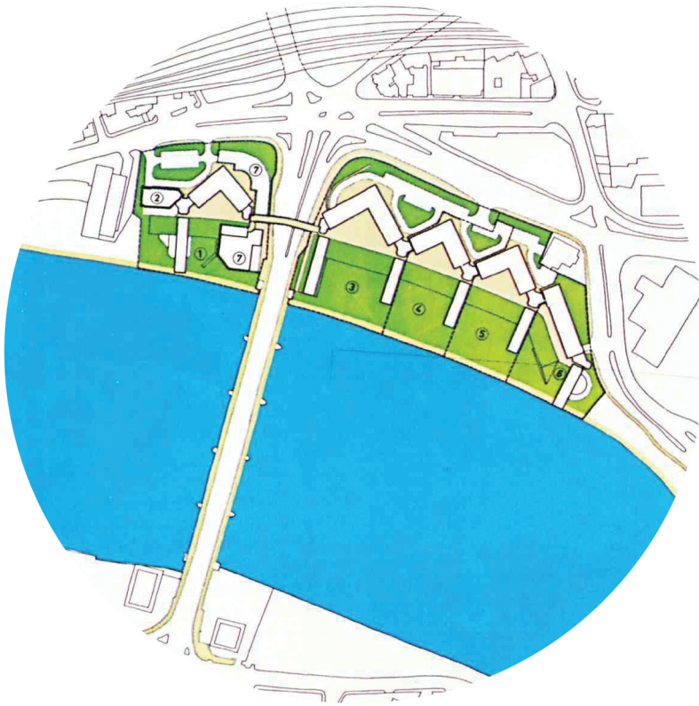
Figure 3. Plan of Sebire Allsopp & Happold's winning entry for the 1981 Arunbridge competition that sought to redevelop the combined Esso and Effra sites at Vauxhall Cross. Sebire Allsopp & Happold's scheme proposed a zig-zag wall of offices to the rear of the site from which stacks of flats stepped down to the riverfront. In the re-entrants of the office zig-zags, the team placed a series of glazed atria that house the public amenity of the brief. Source: Architectural Review 172, no. 1026 (August 1982), 19.
