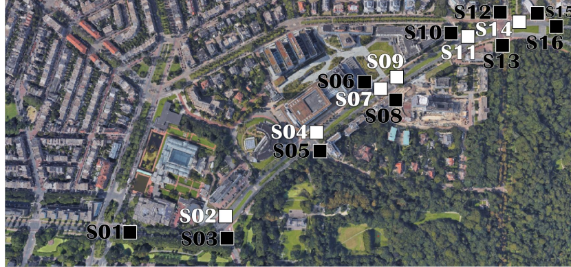
Fig. 1. Layout of the sensors on the S200 road stretch (aerial view).
