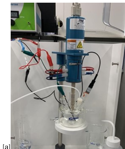
Figure B.4: (a) Photograph and (b) schematic of the RDE setup used for experiments.
