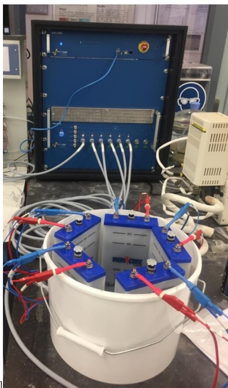
Figure B.5: (a) Photograph of the (a) Battery charging setup and (b) commercial Ni-Fe IronCore batteries used for experiments.
