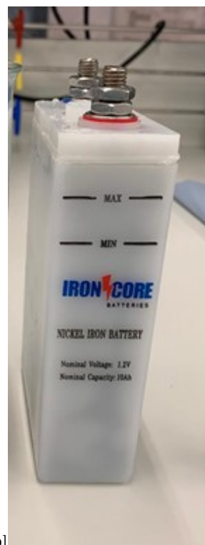
Figure B.5: (a) Photograph of the (a) Battery charging setup and (b) commercial Ni-Fe IronCore batteries used for experiments.
