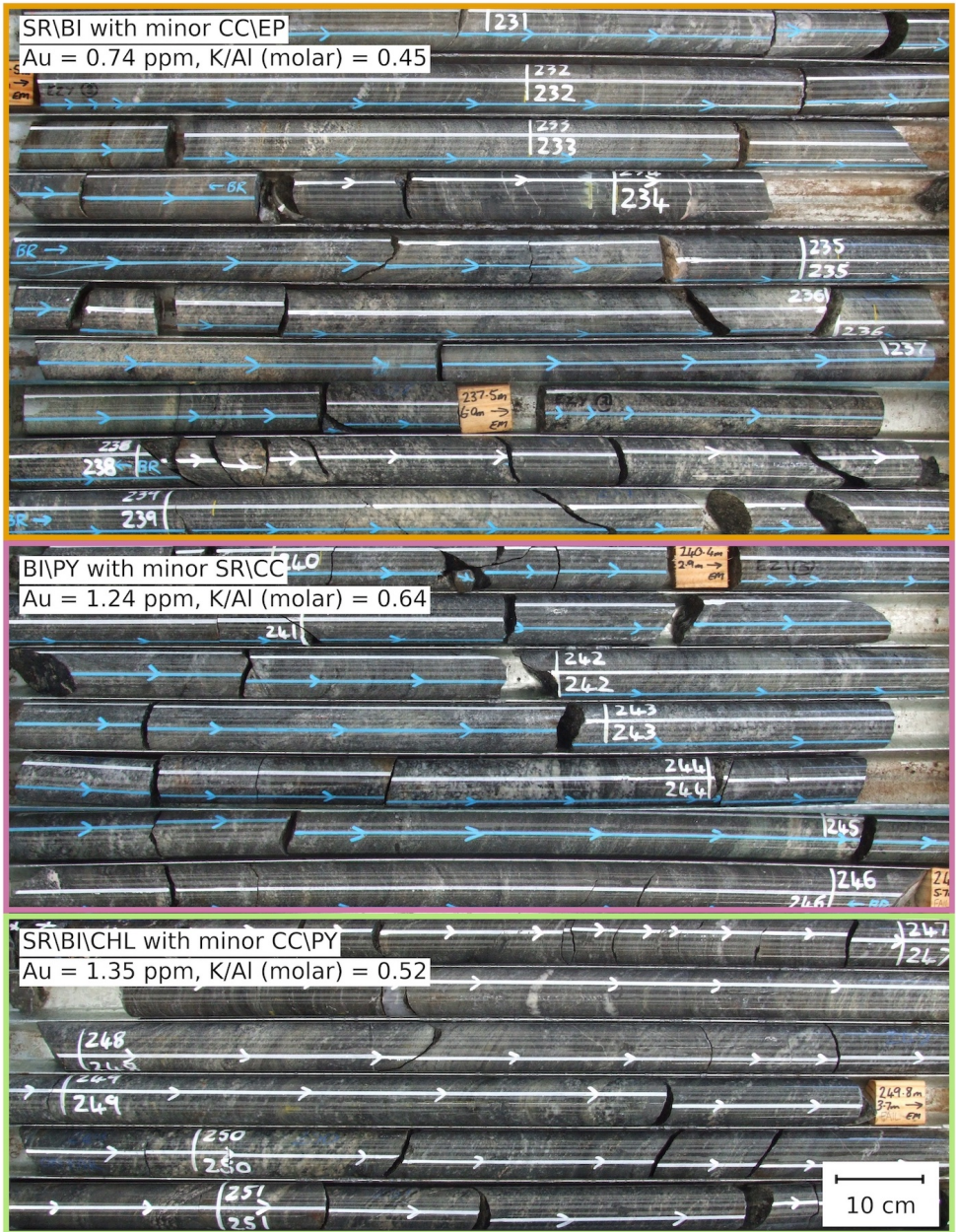
FIGURE 6.8: Core tray photographs of plagioclase (lower molar K/Al) and perthitic K-feldspar rich (higher molar K/Al) feldspathic gneiss domains with distinct zones of alteration. SR: sericite, BI: biotite, PY: pyrite, CHL: chlorite, CC: calcite, EP: epidote. Drill hole TPD234.
