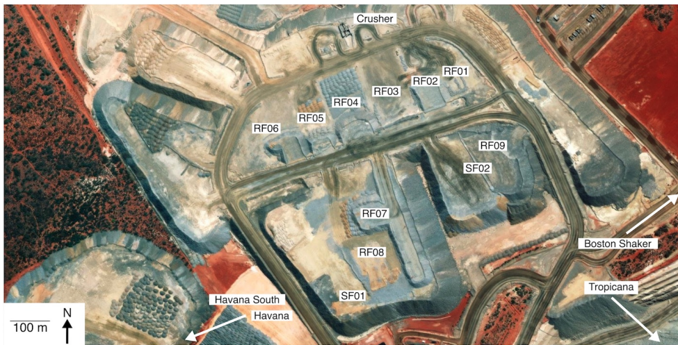
FIGURE 10.6: Aerial photo of the ROM stockpile layout. Note that the layout and location of ROM fingers changes over time. Date: 12 September 2018, (ESRI, 2009).
