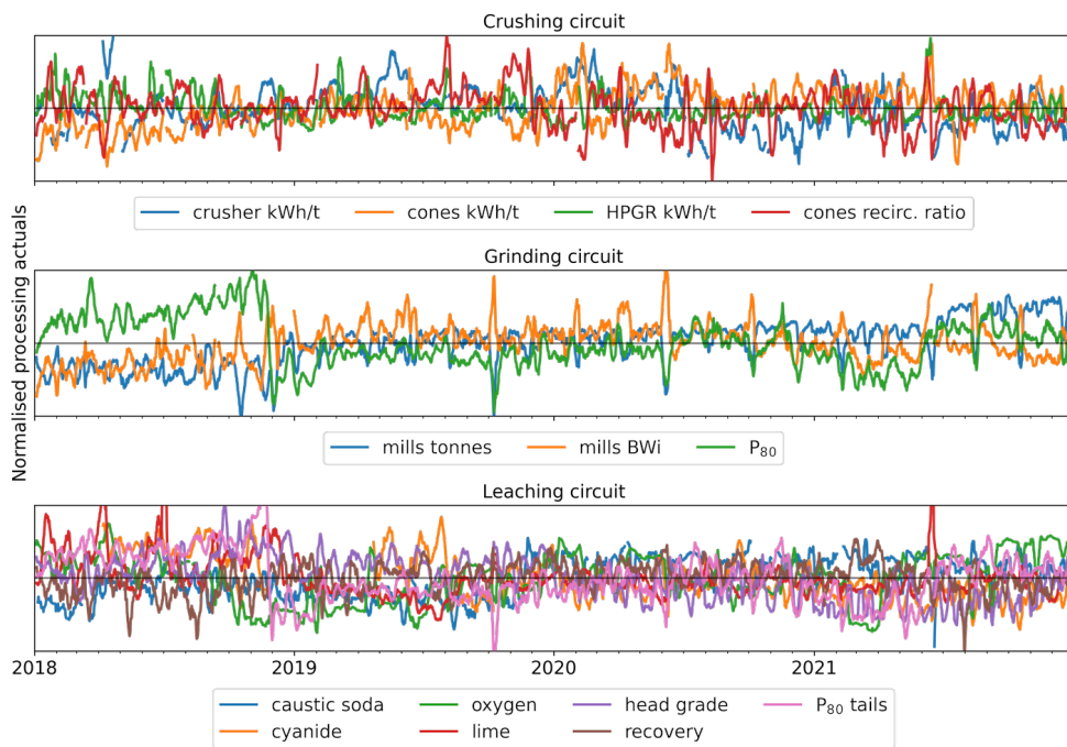
FIGURE 11.3: Time series data visualisation of the seven-day moving averages for selected processing performance indicators.
