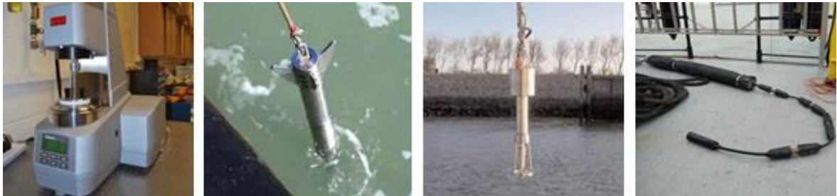
Figure 7: Examples of rheology-based methods. From left to right: lab rheometer (Anton Paar), free falling cone (Graviprobe), tuning fork (Rheotune), towing object (Rheocable)
