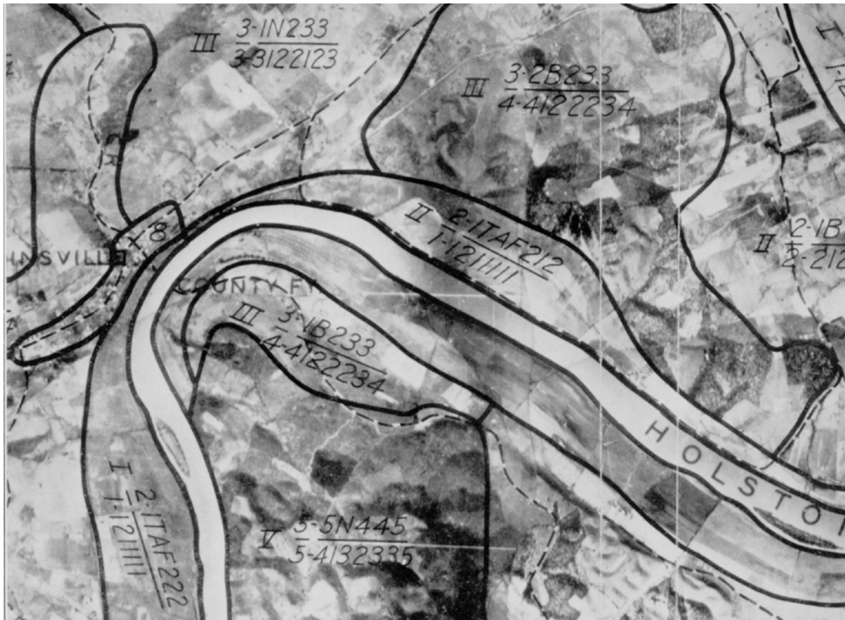
Fig 3.13 Excerpt of TVA survey map Drawn on an aerial photographic mosaic, the map shows the units and the notations describing their characteristics as noted during the field survey. The numerical (so-called fractal ) code indicating particular physical characteristics of the surveyed area allowed the TVA to identify the use of marginal lands and determine broader regional planning interventions such as the treatment of soils, forest conservation or the location of new towns. Hudson (1936), Fig-1.
