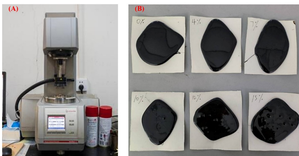
Figure 7. (A) DSR instrument; (B) modified asphalt specimens with different dosage.
