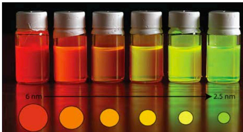
Figure 1.6 Photograph of CdSe quantum dots of different sizes under UV illumination, demonstrating the size tunable emission wavelength. This figure is taken from the ERC starting grant proposal “Doping on Demand”, 2015. 66
