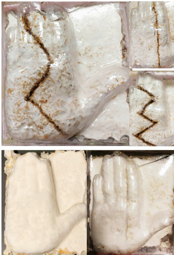
Figure 6. From top left clock wise: 3 different cuts. Then the healed composite after 5 days inside the mould. Lastly the fully healed sample.
