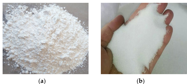
Figure 1. Glass particles: (a) glass powder; (b) glass beads.
