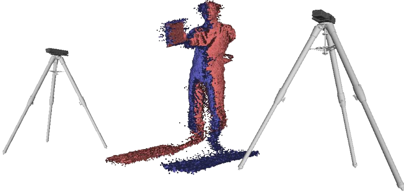
Figure 5.4: Setup of the dual Kinect capturing system. A board is scanned for calibration. The blue/red point clouds are scanned by two Kinect separately. (3D models of the Kinect and the tripod are downloaded from GrabCAD.com , uploaded by Tommi Sintonen and Casey Rayback respectively.)
