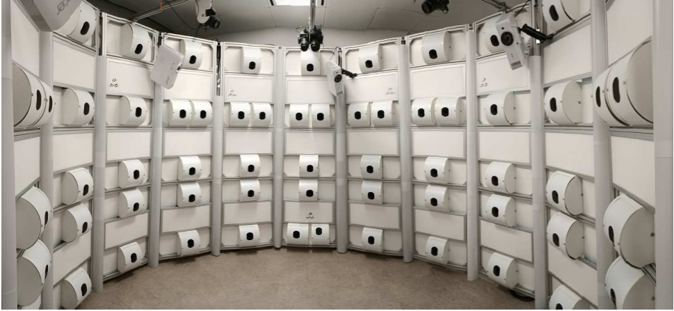
Figure 5.2: Inside of botscan PRO S. More than 70 digital single-lens reflex (DSLR) cameras capture the scene (e.g., a human) inside the scanner from different viewpoints. This is a stitched panorama photo with distortions.
