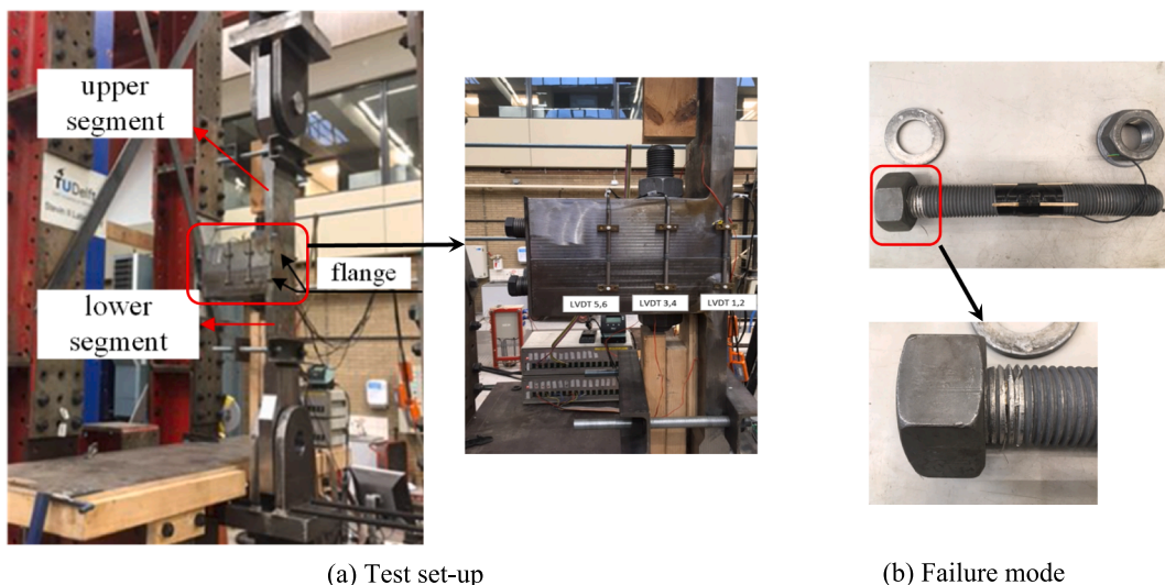
Fig. 6. Test set-up and failure mode for RF connections under static loads.
