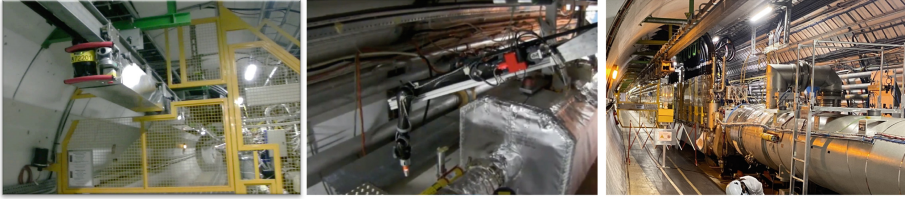
Fig. 2. The TIM robot in the LHC (left), the robotic wagon when the arm is deployed (middle) and obstacles that may not be modeled (right).
