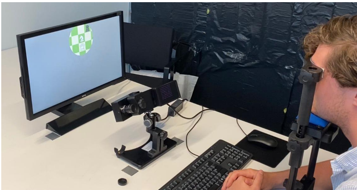
Figure 1. The experimental setup during the memorization phase of the reconstruction task. A gaze-contingent window with a radius of 4.4° is visible on the computer screen.
