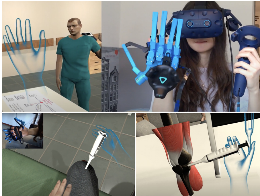
Figure 22.3 Use SenseGlove with HTC Vive tracker to position the hands in VR spaces and train the patient to use an injection tool. SenseGlove can track the fingers, hand, and wrist of user’s hand gestures, and provides force feedback on fingers.
