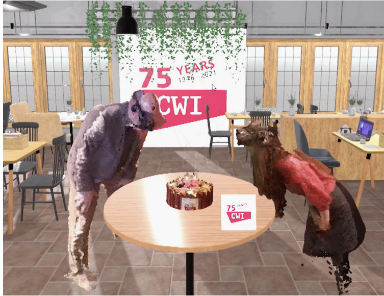
Figure 22.9 Two persons and a cake were recorded in separate locations using three Kinect depth cameras. Their real-time volumetric videos were transmitted into a virtual café so that the two people felt that they were celebrating together.
