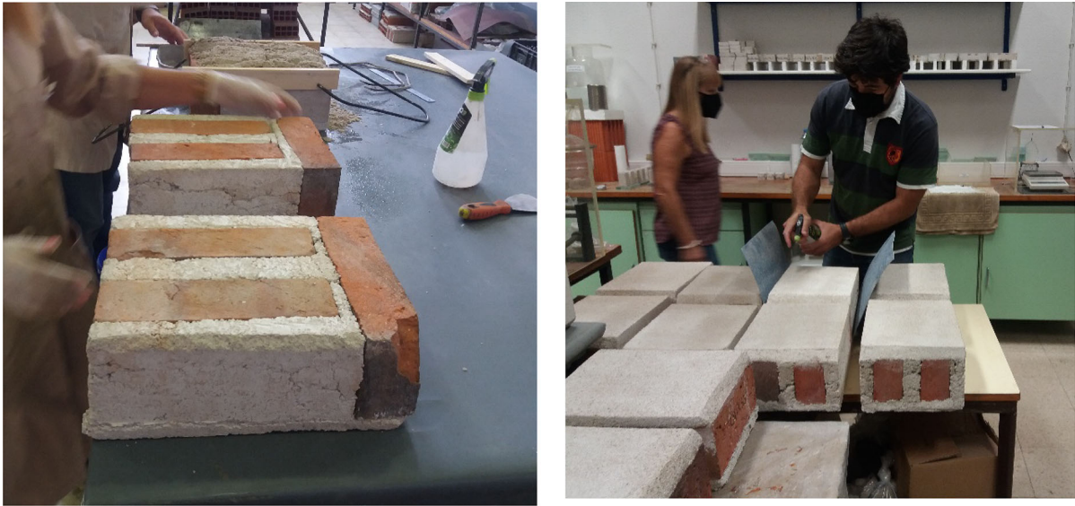
Fig. 16 Porous composite substrates of ceramic brick and lime mortar and application of lime mortar on them
