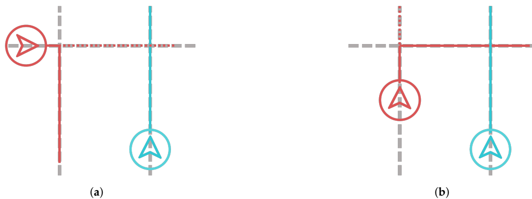
Figure 7. Situations in which a state-based conflict detection method is considered unsuitable: (a) False-positive conflict, blue aircraft detects a conflict based on a linear extrapolation of the current state of the red aircraft; (b) False-negative conflict, blue aircraft has no knowledge of the future turn of the red aircraft, and cannot anticipate the conflict.
