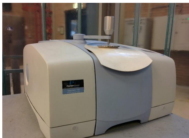
Figure 5-4 TM 100 Optical ATR-FTIR spectrometer
