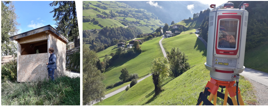
Figure 1.2: Left: the automated total station for geodetic monitoring and its protective housing in Wattenberg, opposite to Vögelsberg (see Figure 1.1), with the author for scale. Right: campaign based laser scanning of the deformation at the Vögelsberg landslide. A technique also applied elsewhere by the Austrian team (Pfeiffer et al., 2018, 2019). Not shown are the unmanned aerial laser scanning campaigns (Zieher et al., 2019). (Images courtesy of Roderik Lindenbergh, October 2018.)
