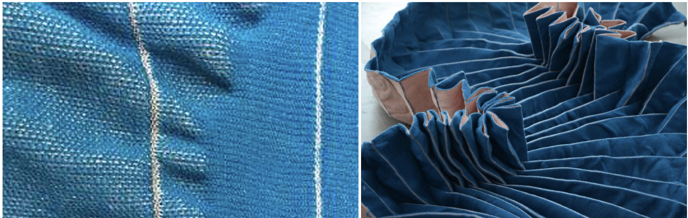
Figure 6: Dynamic Folding Knits by Victoria Salmon [151] is an example of a morphyic textile-form that changes in design/production-time. The density of the knit structure is transformed (left) when heat is applied to the thermoplastic yarn used. This stiffens the structure and enables the embedded folds (right) to activate. Image credit: Victoria Salmon.
