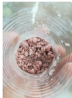
Figure 1: Agglomerated sealant with 5% Al 2 O 3
