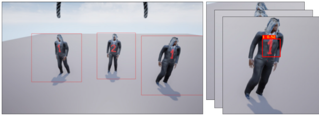
Fig. 4. Pedestrian models, as seen from the drone’s perspective in the realistic environment. Each pedestrian is tracked using AirSim’s API. Its class is represented by a red number in the front, classified using YoloV3.
