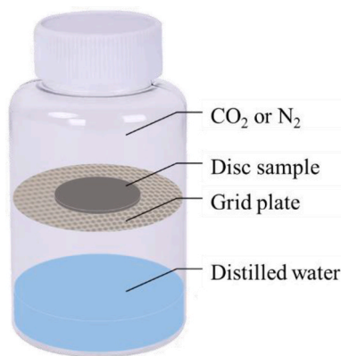
Fig. 2. Schematic diagram of the reaction device for carbonation (CO 2 ) or carbonation free (N 2 ) as the reference.
